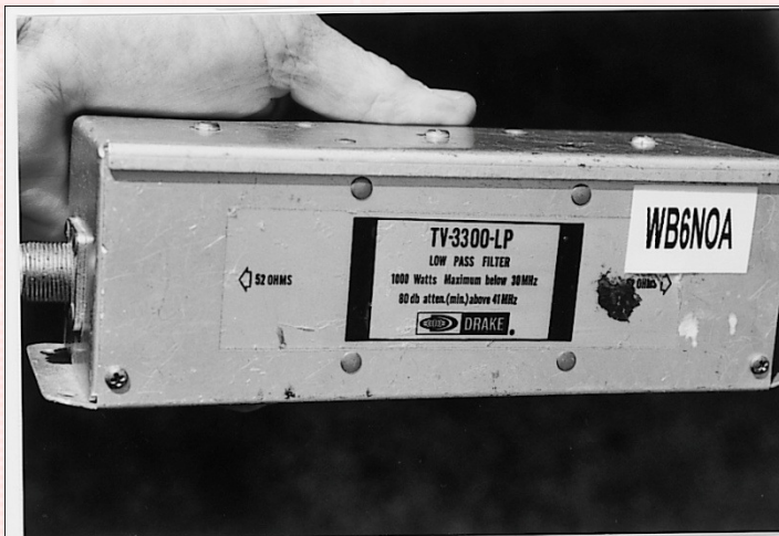
Drake TV-3300-LP Low Pass Filter. 80 db attenuation above 41 MHz. 1000 Watts below 30 MHz.
